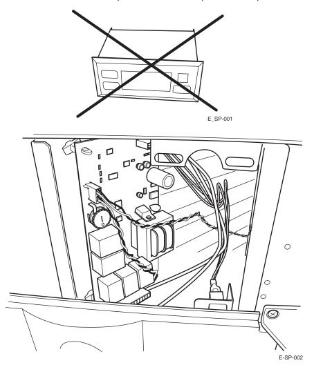
The board is mounted in the lower front section of the CLR2060 Clear Ice Maker and is accessed by removing the service panel.
